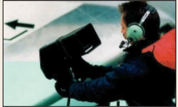
Technical Center has supported the investigation and development of technologies to provide area coverage of ice detection and fluid failure on aircraft surfaces prior to takeoff. The photograph above shows a hand-held system developed with FAA support that is now in operational use.
