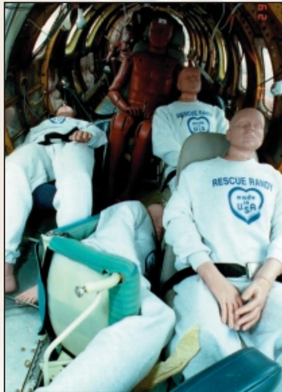
Crashworthy seat design involves two major considerations. First, under high longitudinal crash loads, the seat must not break loose from the floor. Second, under vertical crash loads, the seat must absorb force so that the probability of passenger spinal damage is minimized.
