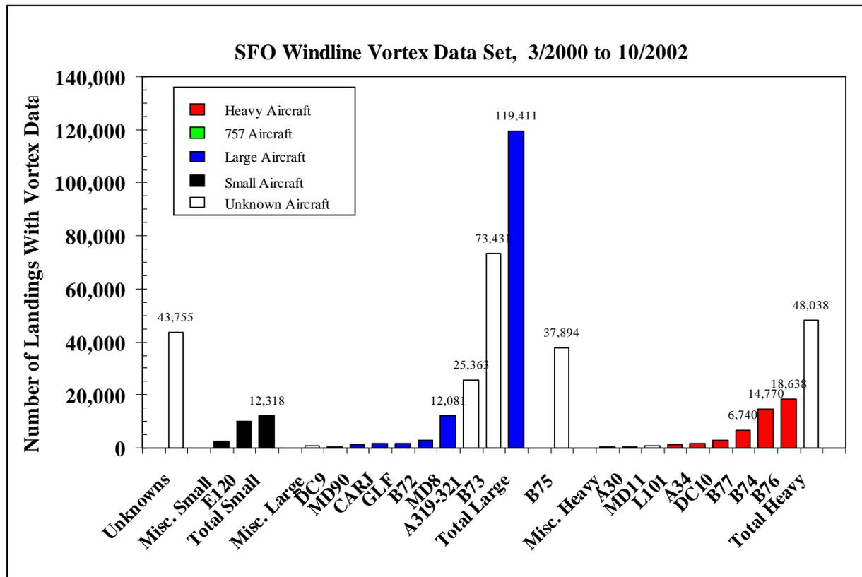
Figure 3. SFO Wake Vortex Landings by Aircraft Type
