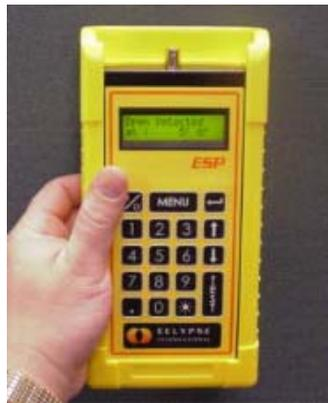
Figure 3. Eclipse ESP Wiring Analyzer
