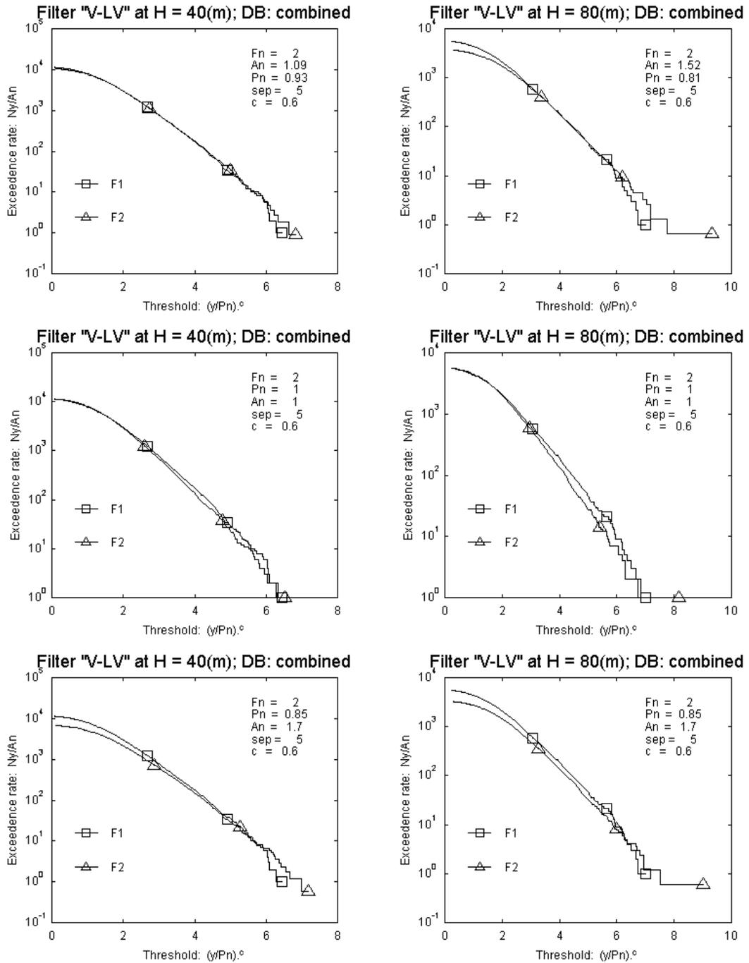
FIGURE A-4. MEASURED STATISTICAL DISTRIBUTIONS ILLUSTRATING METHOD OF MEASURING AMPLITUDE-REDUCTION FACTOR  $P$
