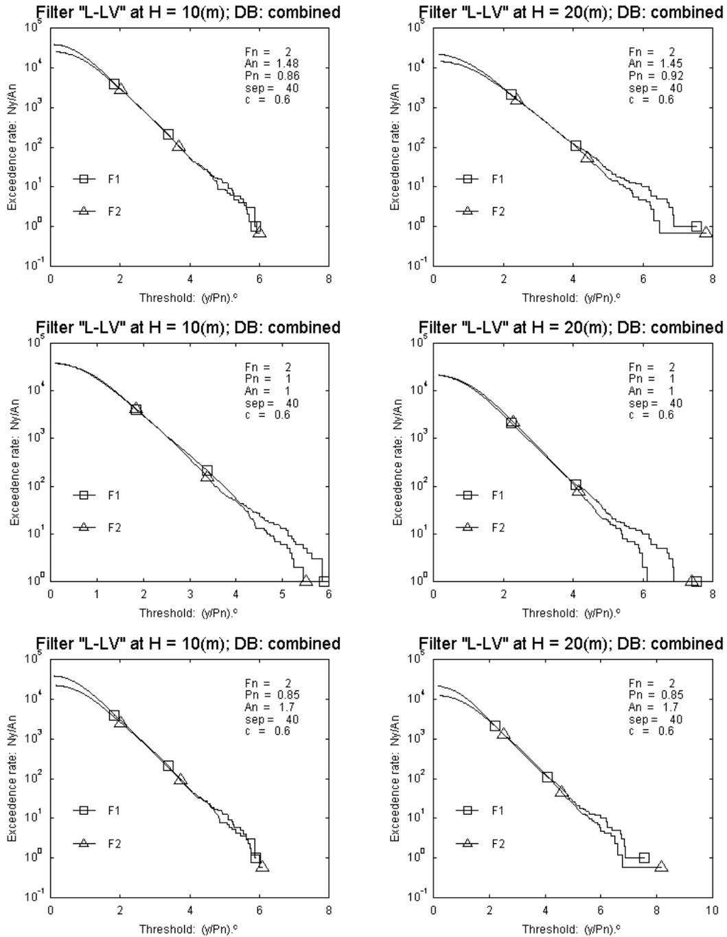
FIGURE A-2. MEASURED STATISTICAL DISTRIBUTIONS ILLUSTRATING METHOD OF MEASURING AMPLITUDE-REDUCTION FACTOR  $P$
