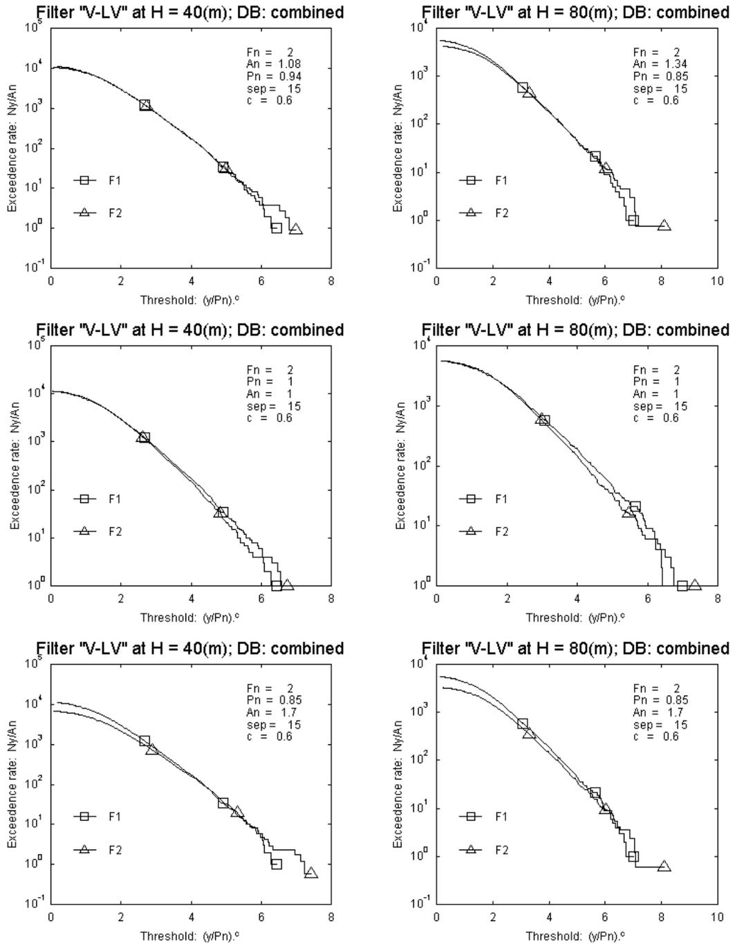
FIGURE A-5. MEASURED STATISTICAL DISTRIBUTIONS ILLUSTRATING METHOD OF MEASURING AMPLITUDE-REDUCTION FACTOR  $P$
