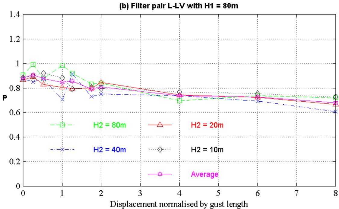
FIGURE 7. MEASURED VALUE OF AMPLITUDE-REDUCTION FACTOR  $P$ , AVERAGED OVER 25 RUNS, INCLUDING GUST COMPONENTS HAVING DIFFERENT GRADIENT DISTANCES,  $H_1 = 80$  m
