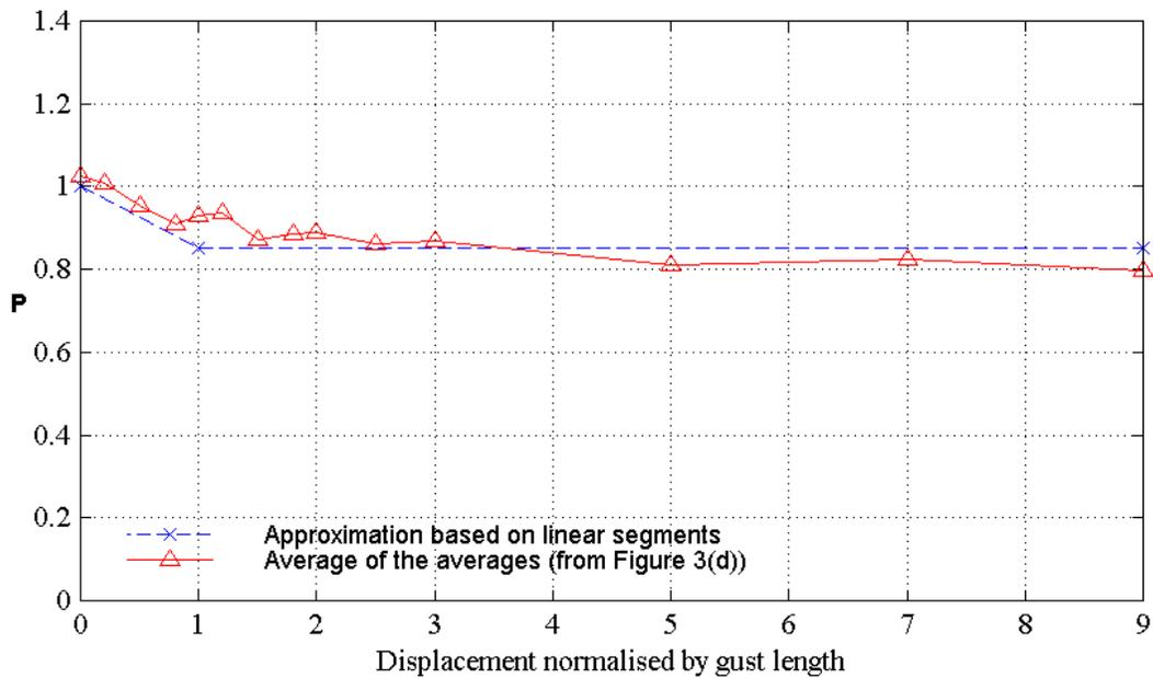
FIGURE 12. APPROXIMATION TO MEASURED AMPLITUDE-REDUCTION FACTOR  $P$  USING LINEAR-SEGMENTS, GUST COMPONENTS HAVING SAME GRADIENT DISTANCE
