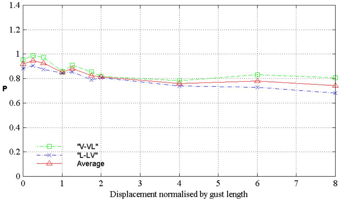
FIGURE 8. MEASURED VALUE OF AMPLITUDE-REDUCTION FACTOR  $P$ , AVERAGED OVER 25 RUNS, INCLUDING GUST COMPONENTS HAVING DIFFERENT GRADIENT DISTANCES. Average of results for  $H1 = 80$  m from figure 7.
