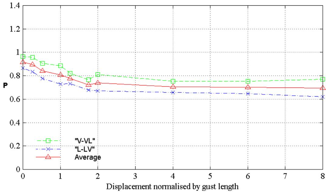
FIGURE 10. MEASURED VALUE OF AMPLITUDE-REDUCTION FACTOR  $P$ , AVERAGED OVER 25 RUNS, INCLUDING GUST COMPONENTS HAVING DIFFERENT GRADIENT DISTANCES. Average of results for  $H1 = 160$  m from figure 9.
