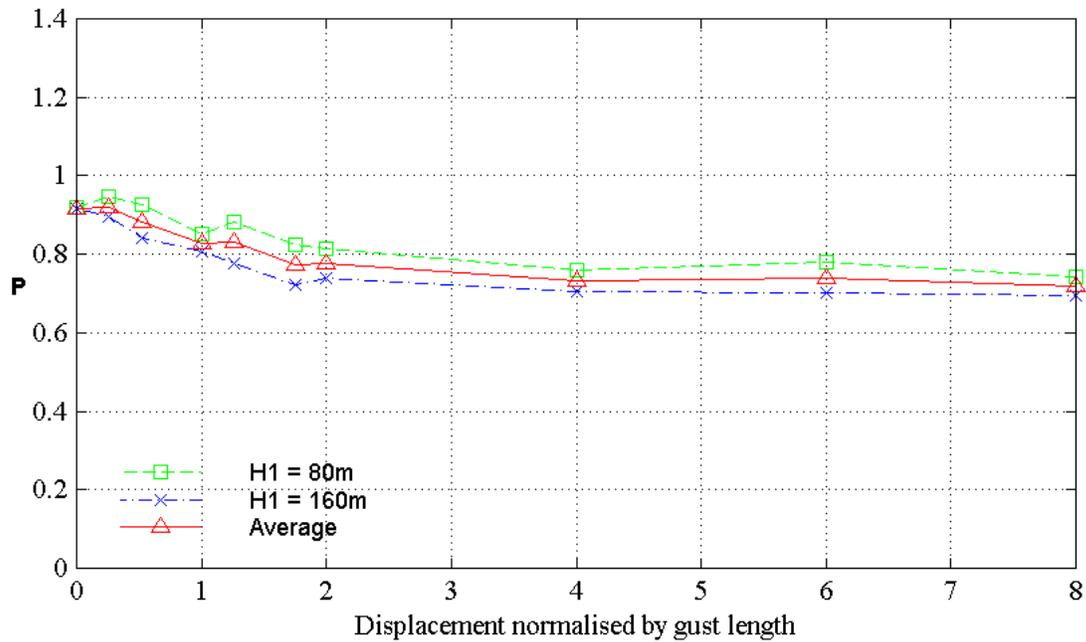
FIGURE 11. MEASURED VALUE OF AMPLITUDE-REDUCTION FACTOR  $P$ , AVERAGED OVER 25 RUNS, INCLUDING GUST COMPONENTS HAVING DIFFERENT GRADIENT DISTANCES. Average of results for  $H1 = 80$  m and  $H1 = 160$  m from figures 8 and 10.
