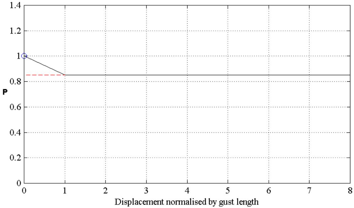
FIGURE 14. RELATIONSHIP BETWEEN LINEAR-SEGMENT APPROXIMATION (SOLID LINE) AND PROPOSED REQUIREMENT INCORPORATING AMPLITUDE-REDUCTION FACTOR  $P$
