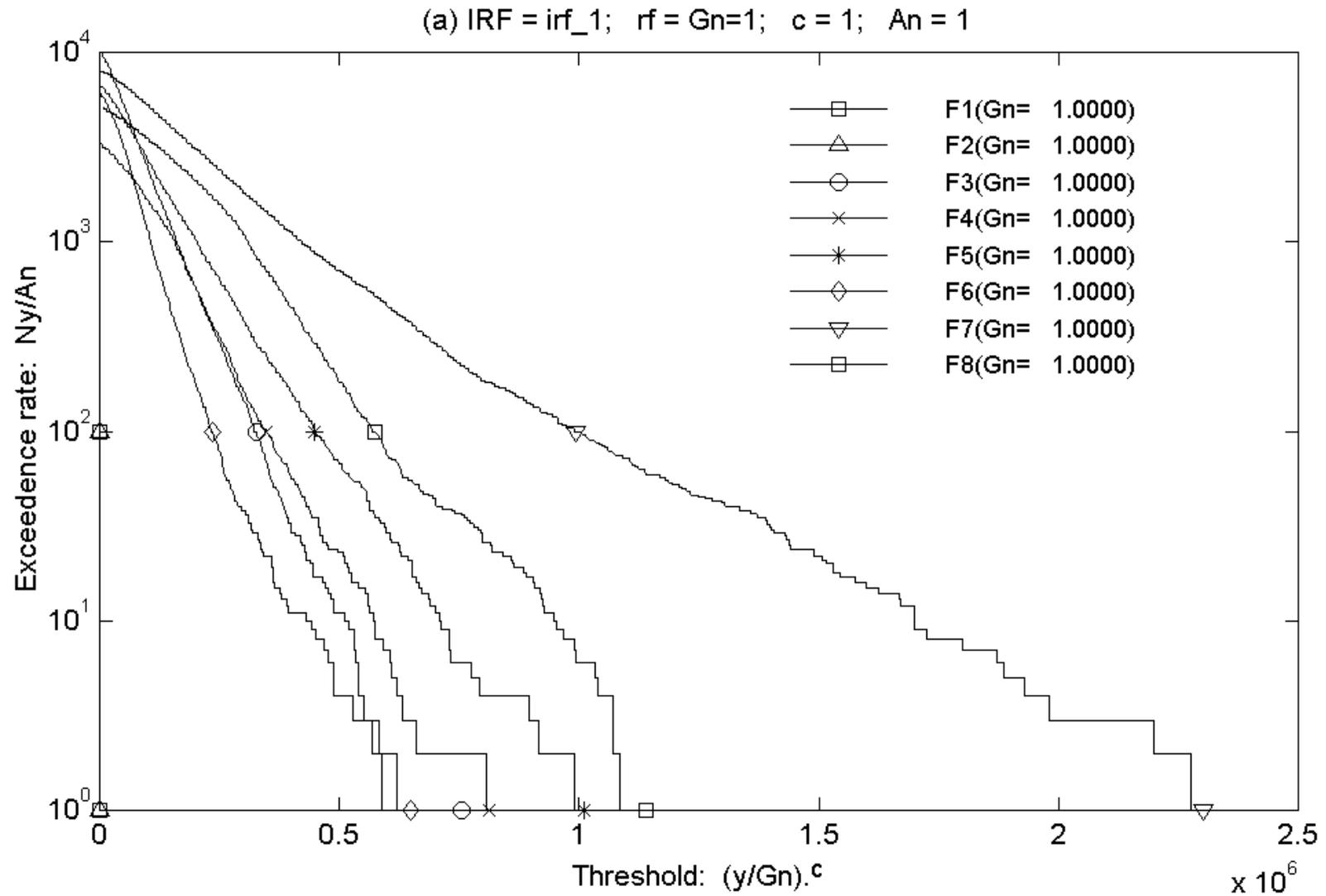
FIGURE 15a. THRESHOLD EXCEEDANCE PLOTS OF RESPONSE TO MULTIAXIS TURBULENCE, FLIGHT CASE 1
