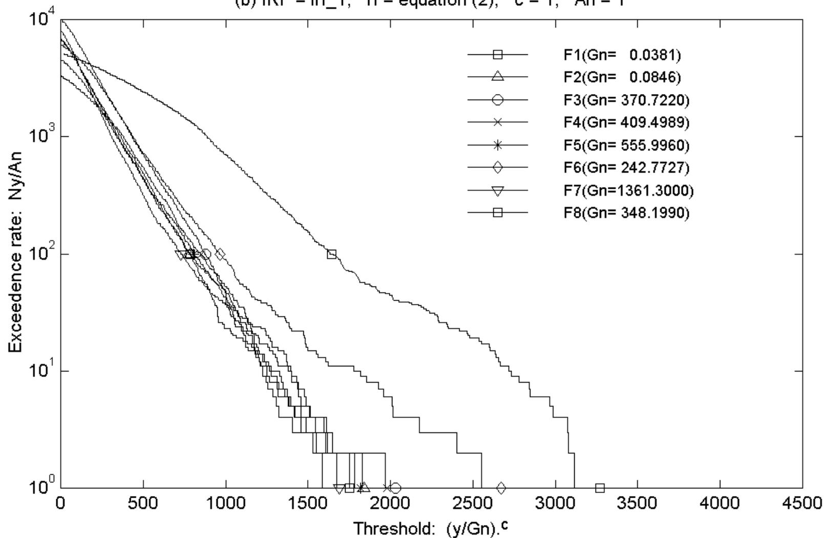
FIGURE 15b. THRESHOLD EXCEEDANCE PLOTS OF RESPONSE TO MULTIAXIS TURBULENCE, FLIGHT CASE 1 PLOTS NORMALISED USING EQUATION 2
