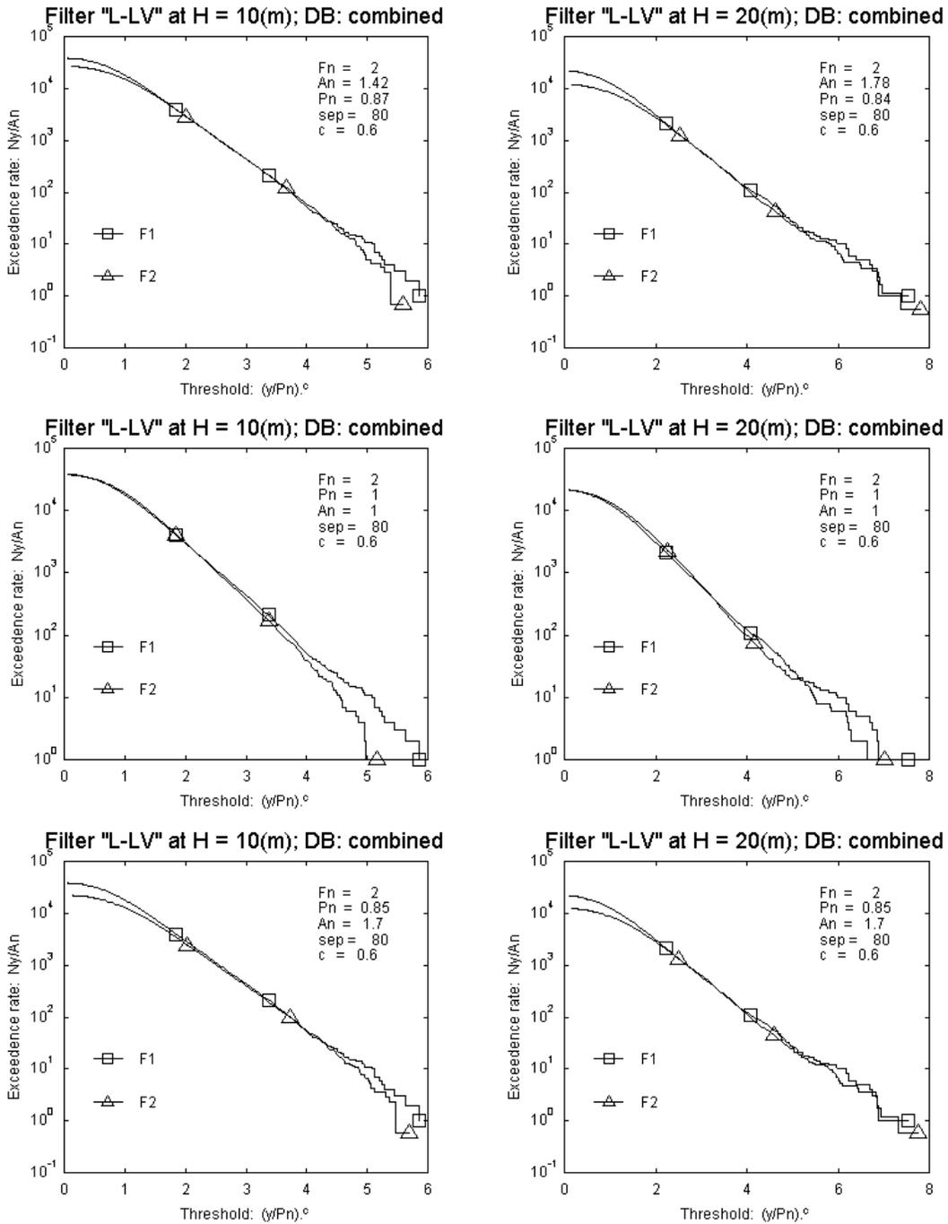
FIGURE A-3. MEASURED STATISTICAL DISTRIBUTIONS ILLUSTRATING METHOD OF MEASURING AMPLITUDE-REDUCTION FACTOR  $P$
