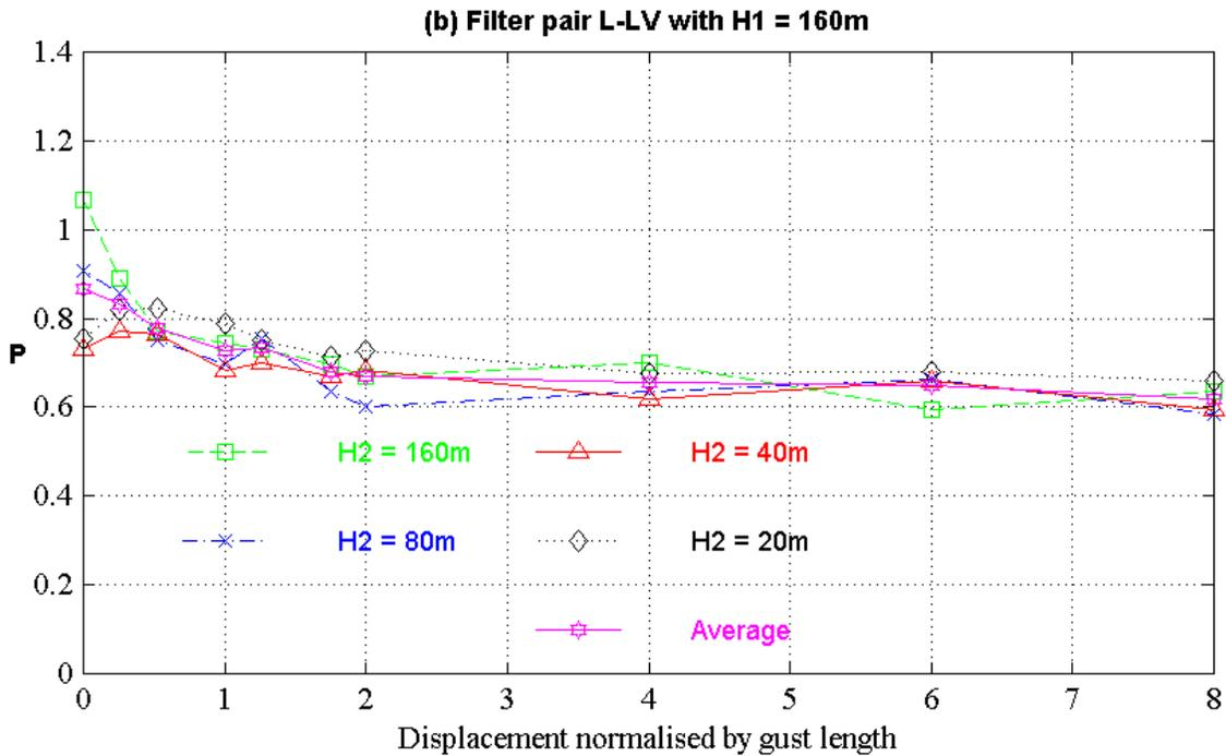
FIGURE 9. MEASURED VALUE OF AMPLITUDE-REDUCTION FACTOR  $P$ , AVERAGED OVER 25 RUNS, INCLUDING GUST COMPONENTS HAVING DIFFERENT GRADIENT DISTANCES,  $H_1 = 160$  m
