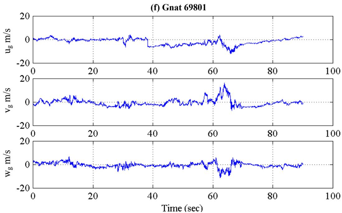
FIGURE 1. EXAMPLES OF THREE COMPONENTS OF TURBULENCE:  $u_g$  (HORIZONTAL),  $v_g$  (LATERAL), AND  $w_g$  (VERTICAL) MEASURED BY GNAT AIRCRAFT (Continued)
