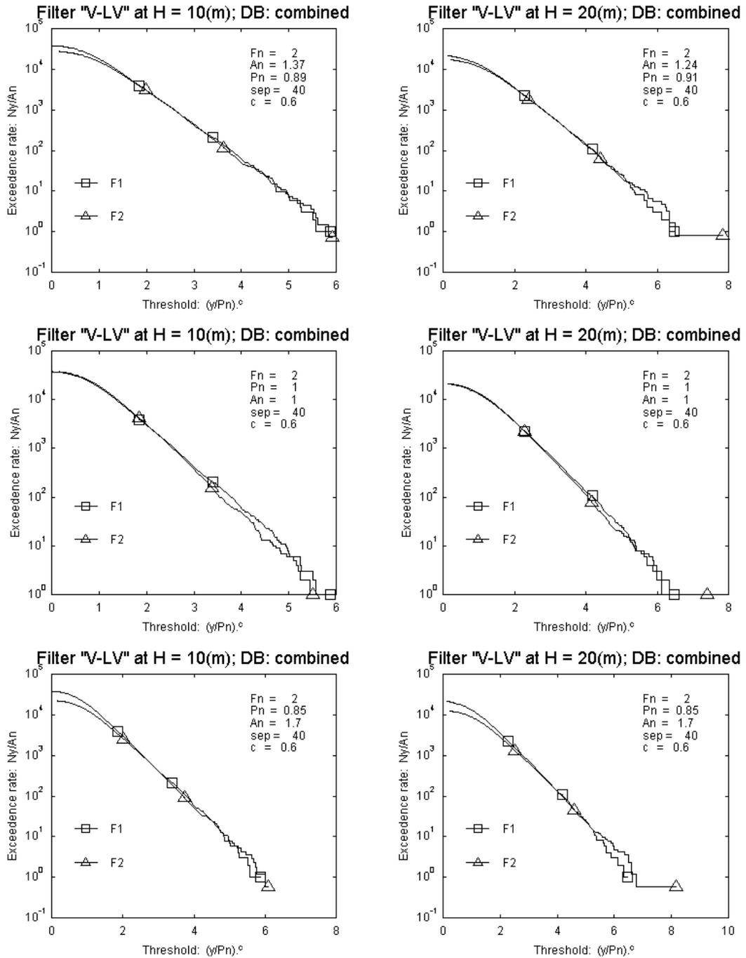
FIGURE A-1. MEASURED STATISTICAL DISTRIBUTIONS ILLUSTRATING METHOD OF MEASURING AMPLITUDE-REDUCTION FACTOR  $P$
