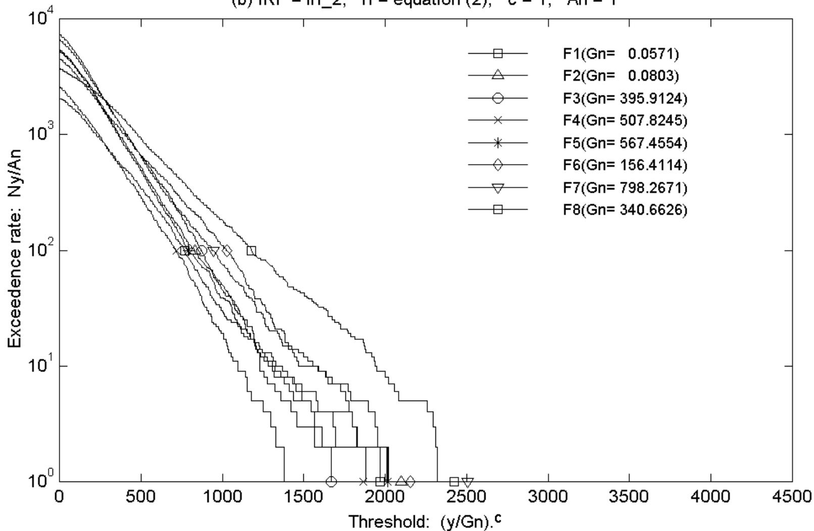
FIGURE 16b. THRESHOLD EXCEEDANCE PLOTS OF RESPONSE TO MULTIAXIS TURBULENCE, FLIGHT CASE 2
