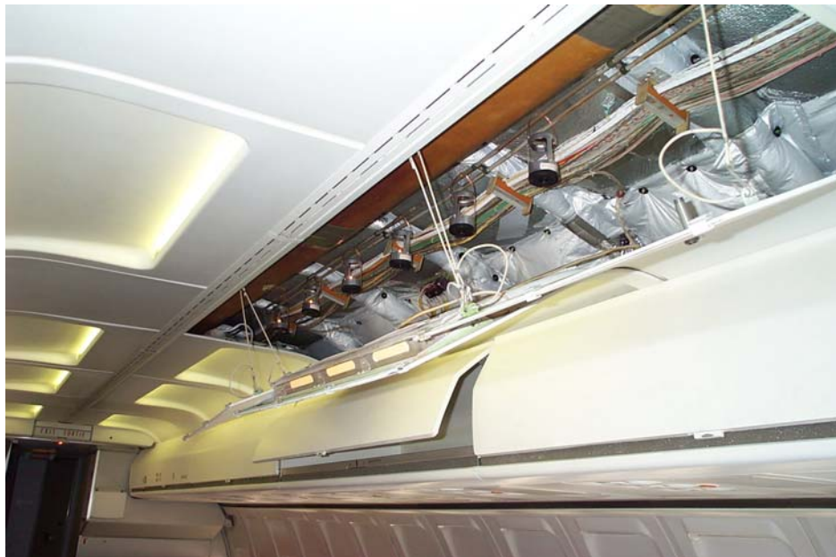
Figure 19. Narrow-Body Aircraft Test Configuration Showing Location of Candle Lanterns
