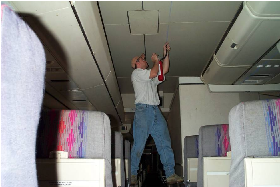
Figure 9. Extinguishing Agent Discharged Through the Port in the Wide-Body Aircraft
