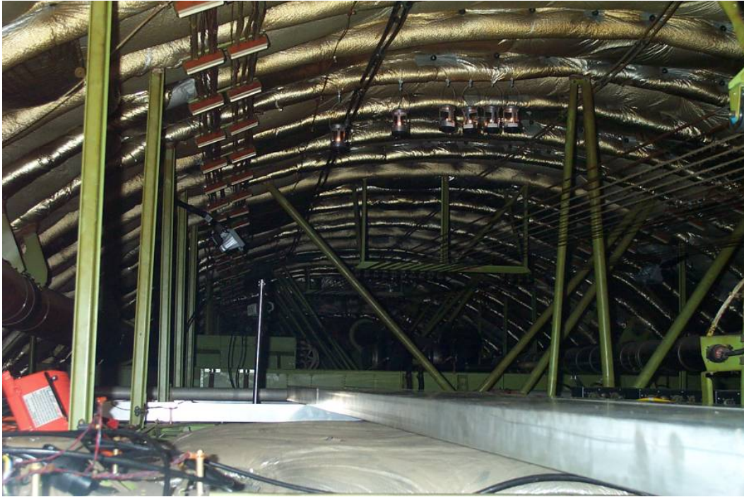
Figure 12. Modified Candle Lantern Test Configuration in Cabin Overhead Area
