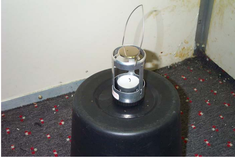
Figure 5. Candle Lanterns Used in Cabin Overhead Area Tests
