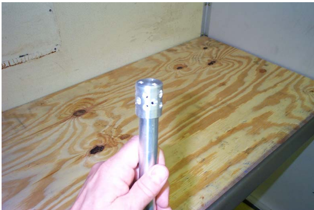
Figure 8. Ceiling-Mounted Port Prototype Discharge Head
