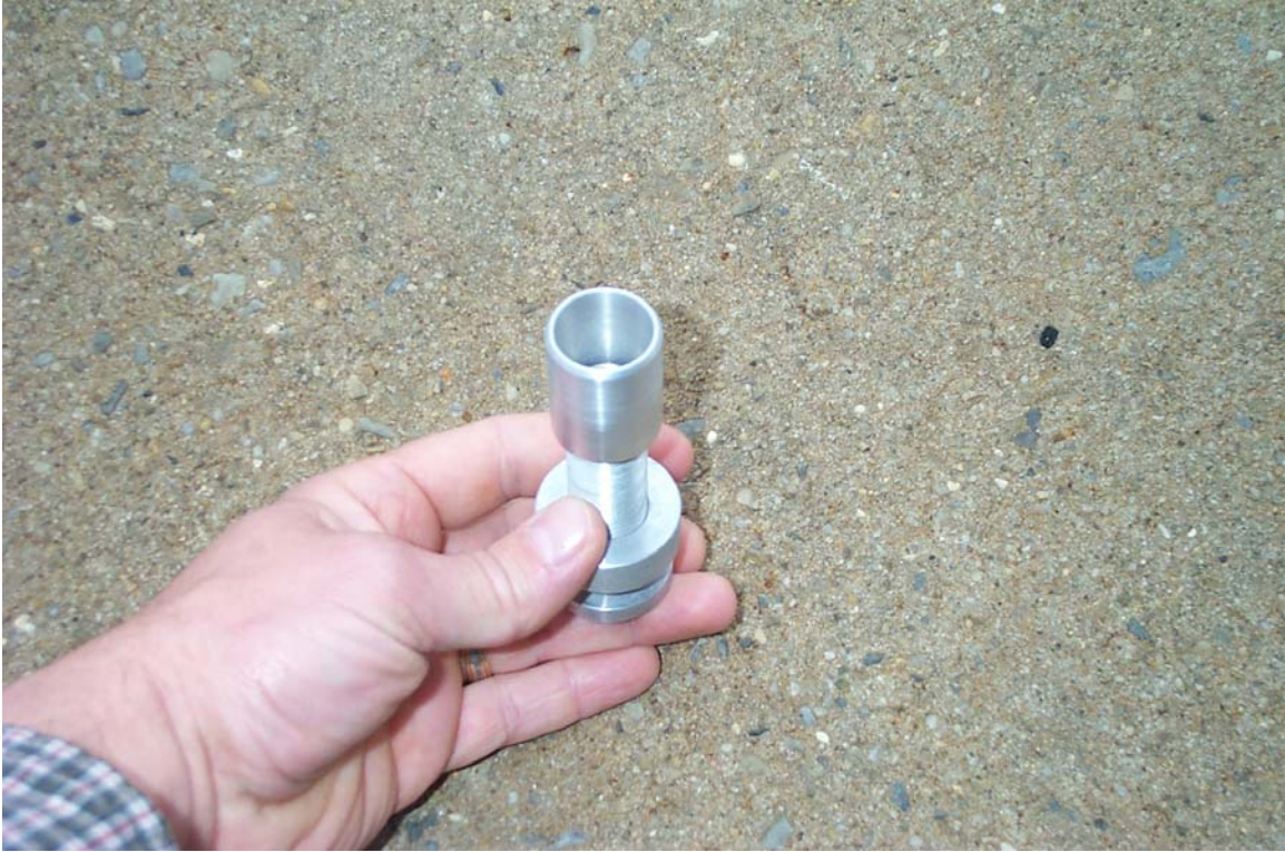
Figure 14. Feedthrough Design Discharge Head
