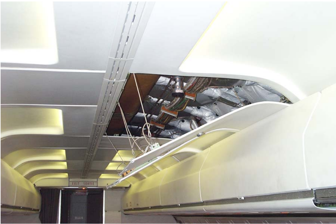
Figure 17. Narrow-Body Aircraft Showing Cabin Overhead Area Access
