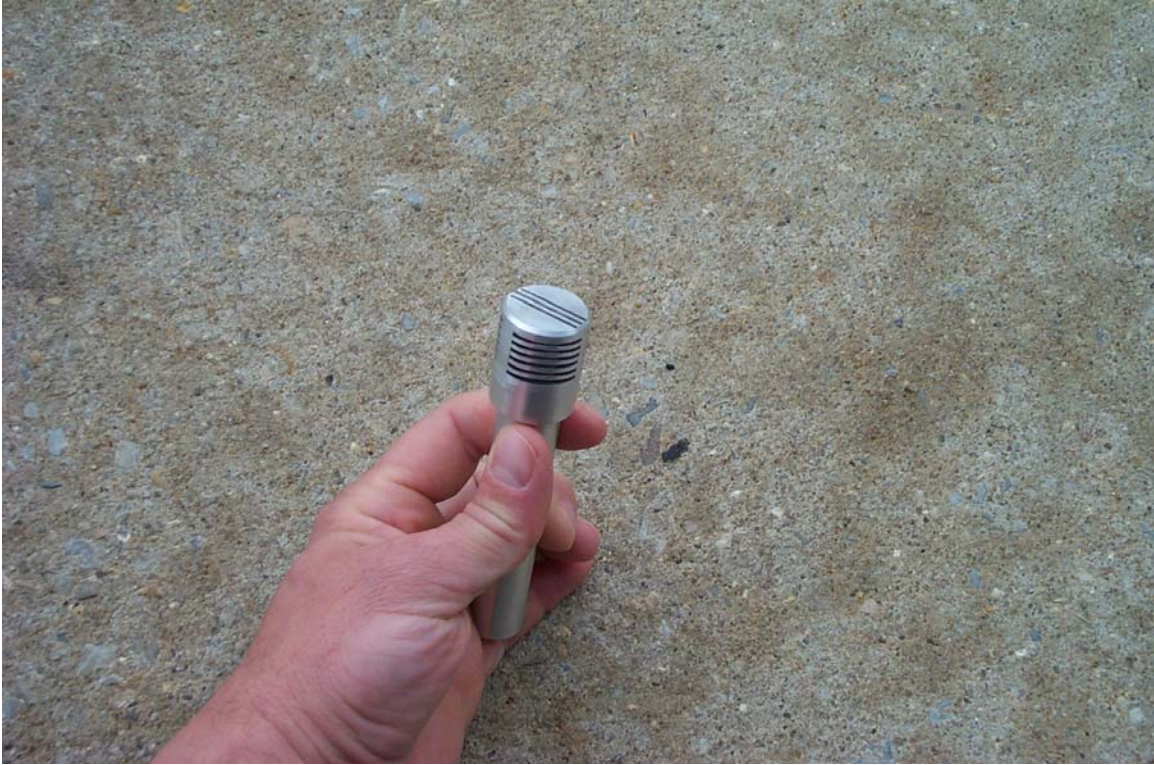
Figure 13. Grill Design Discharge Head
