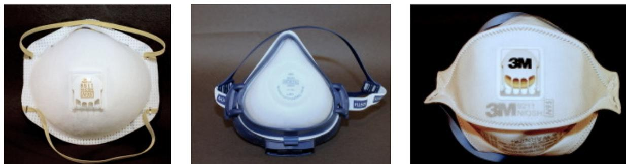
Figure 8. The three N95 respirators (3M™ 8511, North 4200, and 3M™ 9211) tested in Phase 2.
