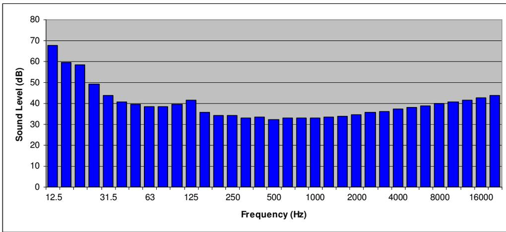
Figure 13. Frequency spectrum of the anechoic chamber.
