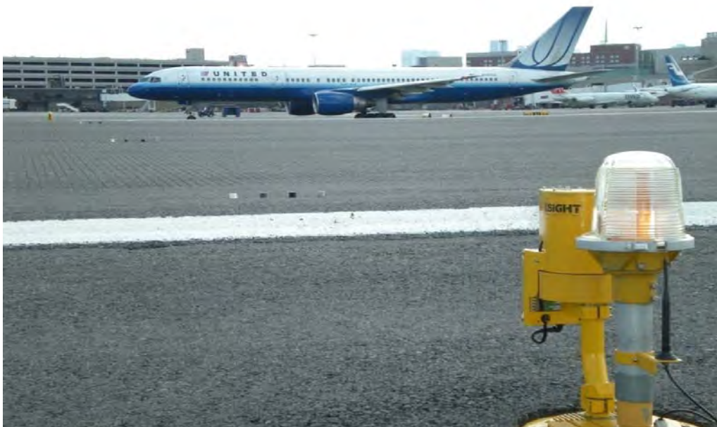
Figure 2. The FODetect Sensor With Targets on the Runway at BOS
