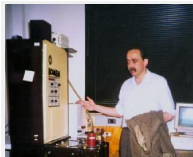
*A high resolution Fourier transform infrared spectrometer. This instrument is used for measuring the infrared signatures of explosives in the solid, liquid and vapor phases and for explosives adsorbed on various surfaces used as collectors in explosive detection systems (Dr. Henderson).*
