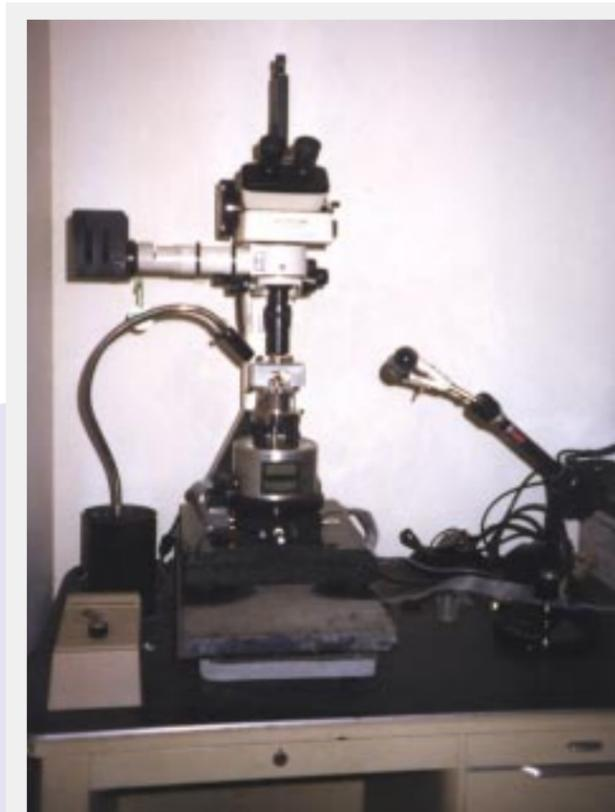
*An atomic force microscope, purchased through an FAA grant, used for imaging nanoparticles of explosives deposited on various substrates.*
