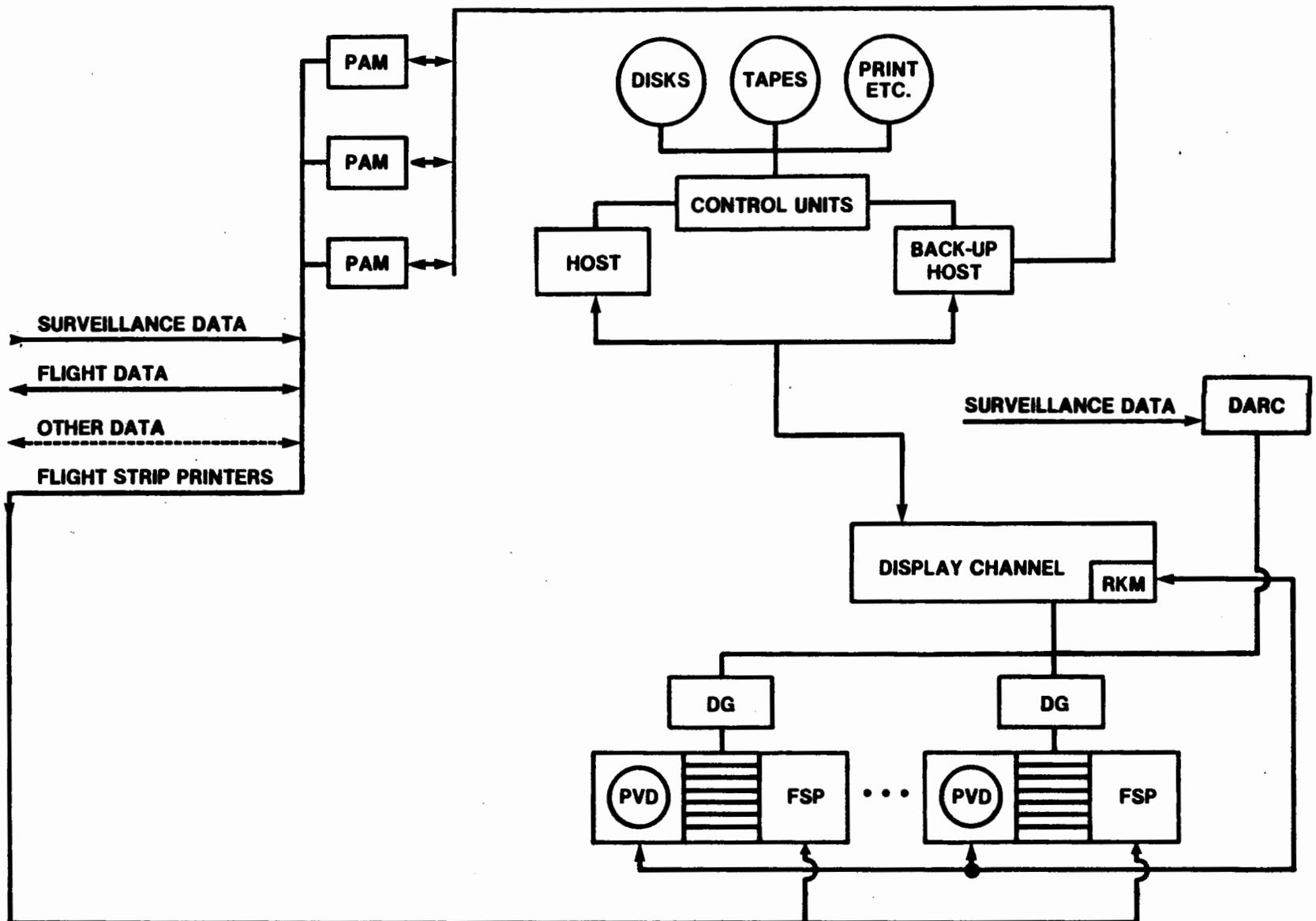
**FIGURE 4: HOST AFTER REMOVING 9020, STATE 1**
