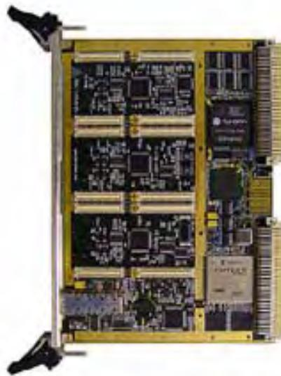
Figure D-17. The VME Detection Processor Card
