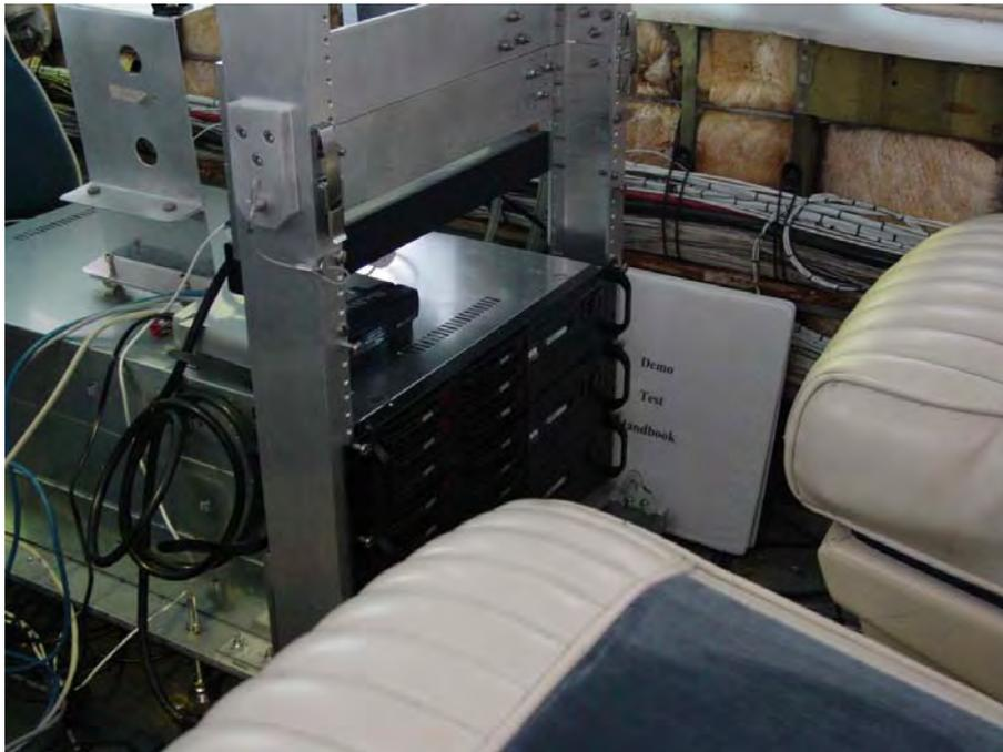
Figure D-5. The ATDSS I Data Recorders and Detection and Tracking Processors in the Aero Commander Cockpit
