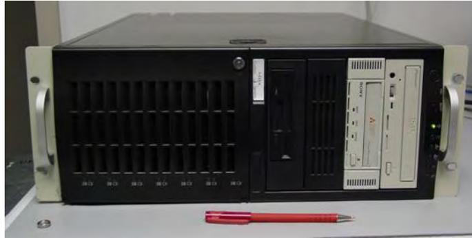
Figure D-12. Chassis Enclosing Detection and Tracking Processors
