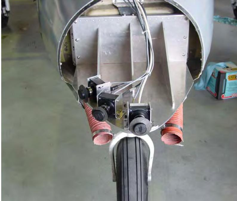
Figure D-4. The ATDSS I Sensor Installation in the Aero Commander
